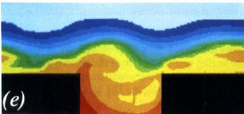
FIGURE 18. A plot of the isotherms (temperature fills) during one flow cycle in the base geometry at  $R = 525, \eta = 0.2, \Omega_F = 0.168 (= \Omega_{n, 1})$  and  $Pr = 1$ . Note the imprint of the Tollmien-Schlichting waves on the resulting temperature distributions. (a)  $\Omega_F t = 0$ ; (b) 0.2; (c) 0.4; (d) 0.6; (e) 0.8.
